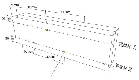
Nail or Bolt sizes in line with specification detailed in relevant STEICO Technical Bulletin
