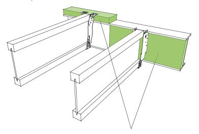
Timber packers and plates to Steel beam designers specification
