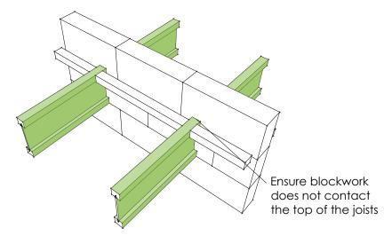
89mm minimum bearing for continuous joists. Ensure discontinuous joists have a minimum 45mm bearing. Joists may be lapped for a full bearing
