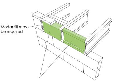
Blockwork may be built up around i-joists or blocking pieces used to restrain the end of the joists
