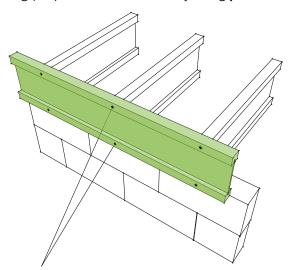
1 No 3.75 nail per flange. Nail length to ensure minimum 35mm embedment depth.
