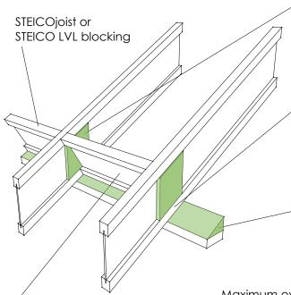
Bevelled web stiffeners may be required both sides of joist
