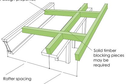
Overhang no greater than the rafter spacing or less than 600mm
