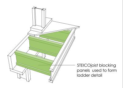
Minimum nailing for class 1 structures to be 3.00\*75 nails at 300mm centers which should be applied at each interface where lateral loads are to be transferred. Refer to STA "Design Guidance on Disproportionate Collapse" for further information
