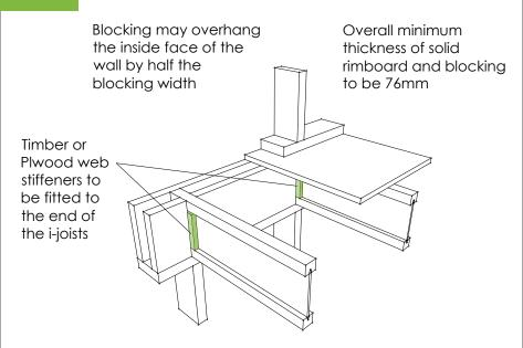
Minimum nailing for class 1 structures to be 3.00\*75 nails at 300mm centers which should be applied at each interface where lateral loads are to be transferred. Refer to STA "Design Guidance on Disproportionate Collapse" for further information
