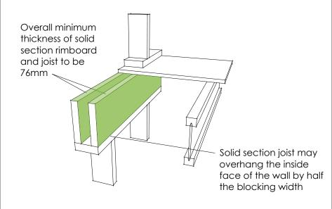
Minimum nailing for class 1 structures to be 3.00\*75 nails at 300mm centers which should be applied at each interface where lateral loads are to be transferred. Refer to STA "Design Guidance on Disproportionate Collapse" for further information
