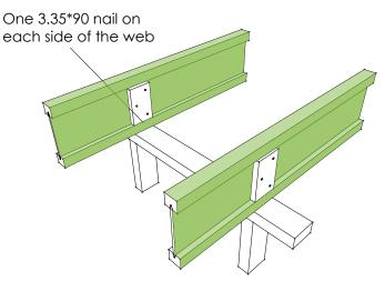
Blocking may be required for sound or fire detailing or where specified by the building designer
