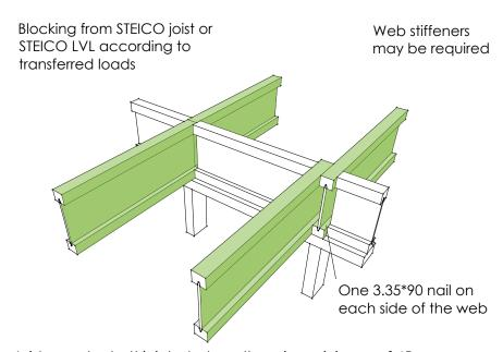
Joists may be butt jointed where there is a minimum of 45mm bearing available. If this is not possible joists are to be staggered and provided with full bearing
